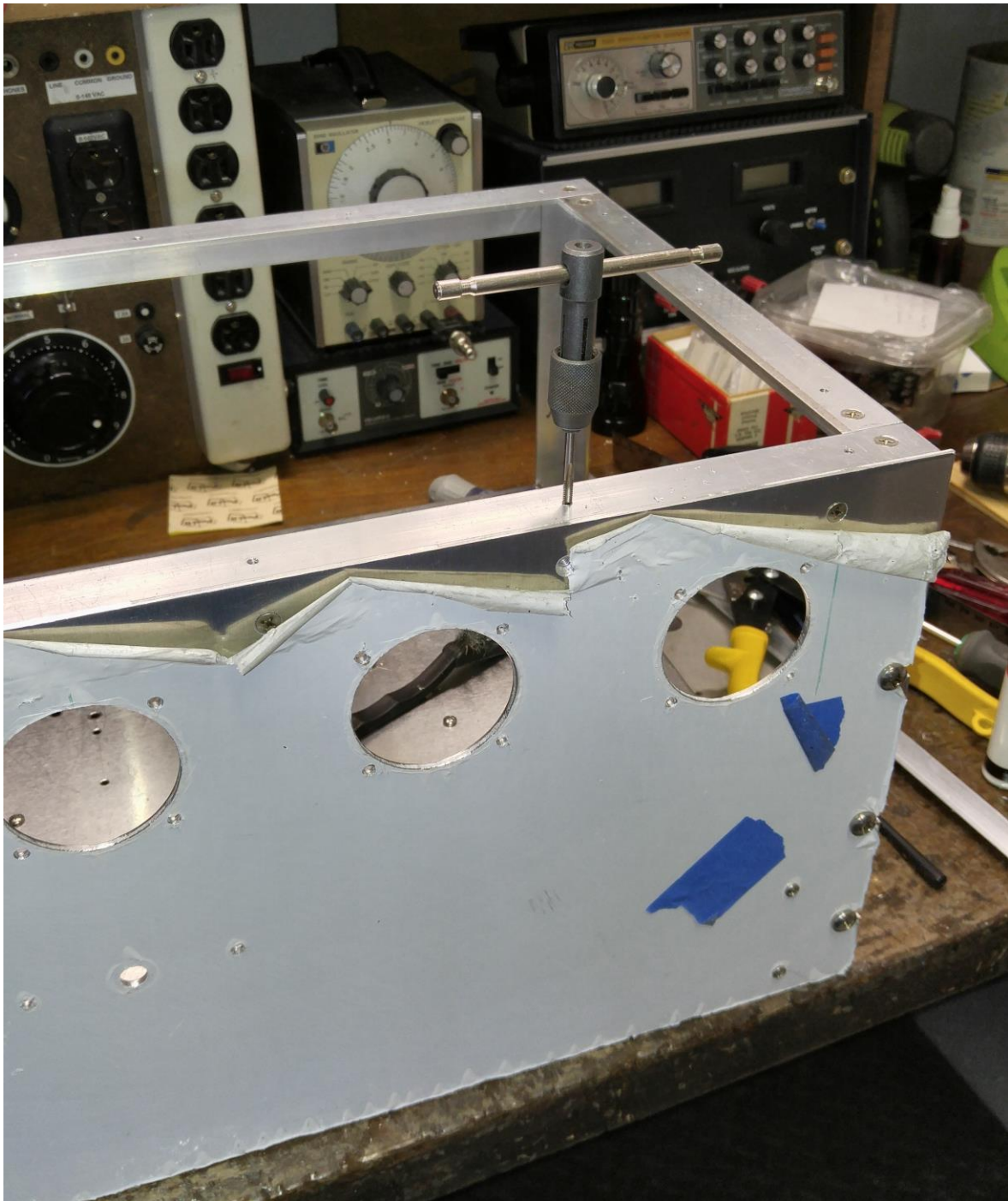
Figure 4: Tapping Holes in Cabinet Frame
