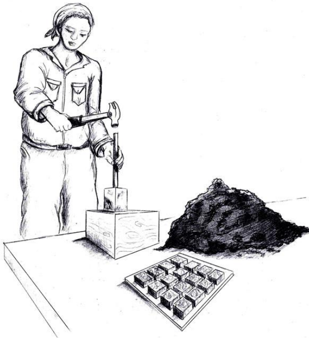
Figure 2-11: Using a briquette press.
