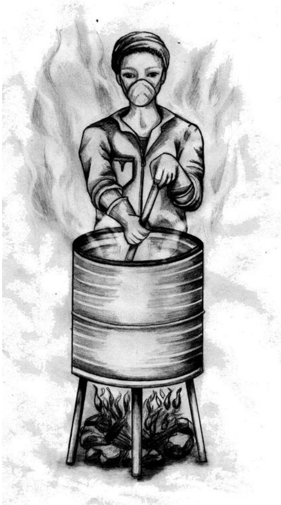
Figure 8-6: Keep mixing the melting plastic until it is a black liquid with no lumps.
