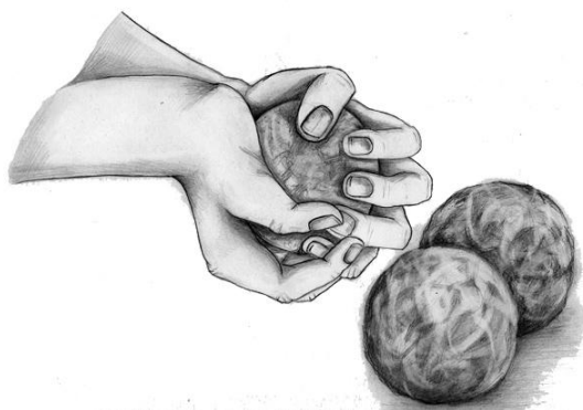
Figure 2-3: Sawdust briquettes can be made by hand, concept by Joyce Lockard.
