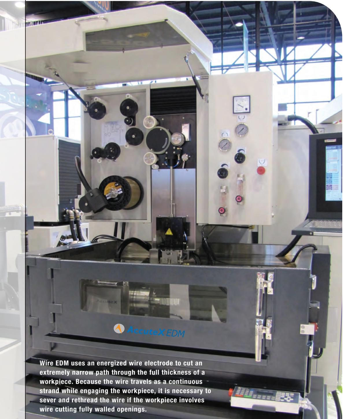
Wire EDM uses an energized wire electrode to cut an extremely narrow path through the full thickness of a workpiece. Because the wire travels as a continuous strand while engaging the workpiece, it is necessary to sever and rethread the wire if the workpiece involves wire cutting fully walled openings.
