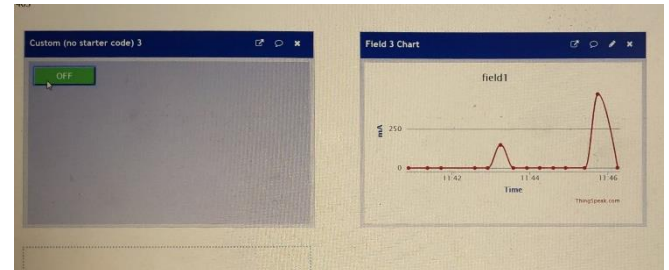
Figure 10: Switch turning of and amount of current consuming by the load plotted on the Things peak Cloud based services.
