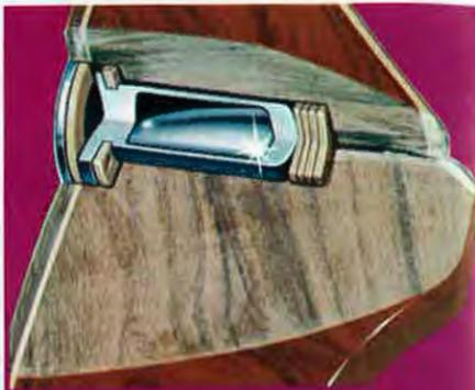
Steel cartridge partly filled with mercury. When the arrow is released and the limbs snap forward, the mercury explodes within each cartridge, then instantly returns to its original form, absorbing vibration and reducing torque.
