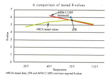
A review of NRCA's test results reveals tested R-values lower than the predicted five-year-old value in laboratory conditions (LTTR = 6.0). Also, NRCA's tested values are somewhat lower than those of ASTM C1289, "Standard Specification for Faced Rigid Cellular Polyisocyanurate Thermal Insulation Board," at 40°F.
