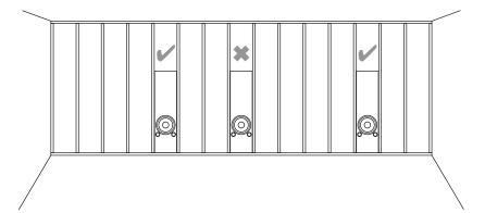
In some situations, it may not be possible to install the subwoofer into a wall. In this case the ceiling, floor, or even a closet are options. Wherever the IW-Basis 300 is installed it must be securely mounted. If it is not securely mounted, its substantial bass output may produce rattles. In addition, be sure that the connectors are accessible for electrical hook-up.
