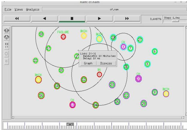
**Fig. 6: Data aggregation at Cluster heads**
