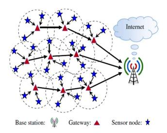
Fig. 1: A Wireless sensor network model
