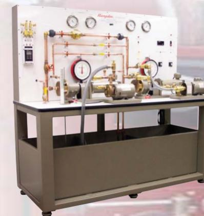
Hampden's Model H-6980 Series/Parallel Pump Test Demonstrator provides two methods of determining flow rate which can be manually adjusted using a throttle valve.
