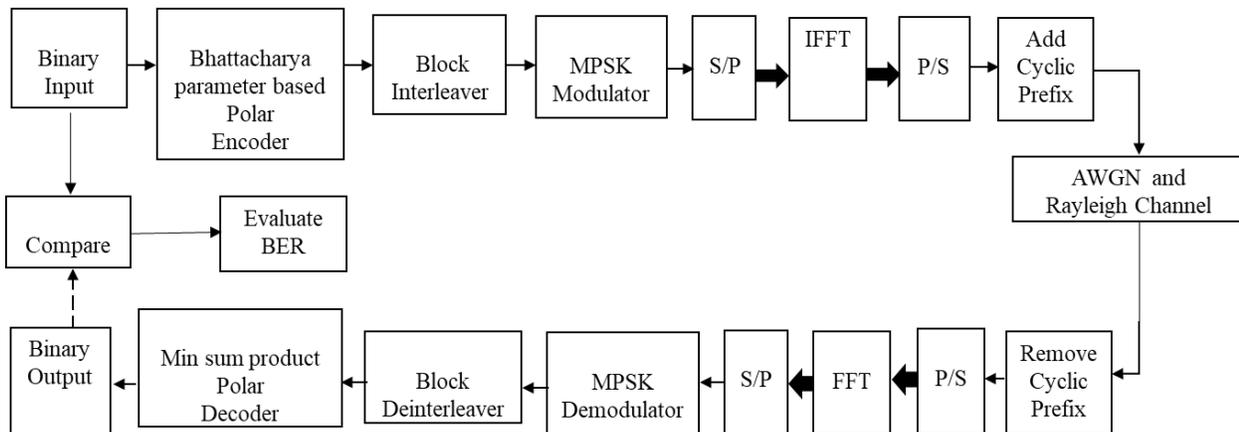
Figure 1. Test Engine Model for simulation of Polar-code Based OFDM-IDMA System
