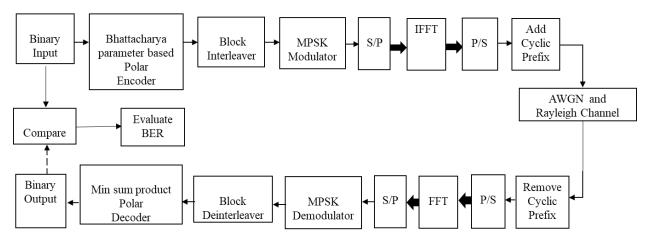
Figure 1. Test Engine Model for simulation of Polar-code Based OFDM-IDMA System
