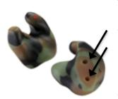
Two parallel sound paths that lead into the sound bore are on the outside of the earplug. Each of these sound paths houses a small orifice filter that limits the attenuation of softer ambient sounds while increasing the
