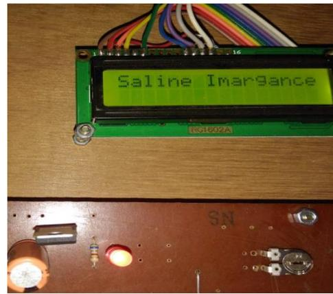
Fig 7. Figure showing Saline emergency on display outside ICU
