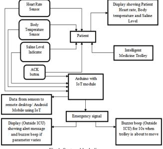
Fig 4. System block diagram
