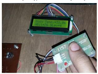
Fig. 6. Figure showing all three parameters that are monitored
