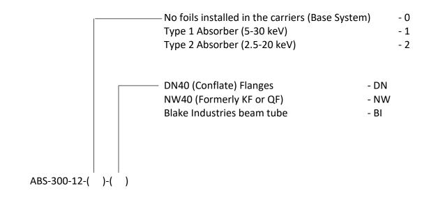
For example, a chamber configured for 5-30 keV with DN40 flanges would be denoted by: ABS-300-12-1-DN
