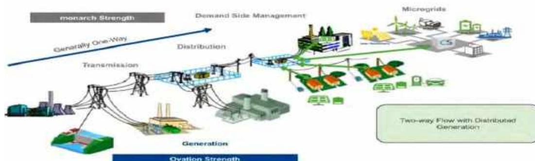
**Fig 1: Two-way Power flow**
