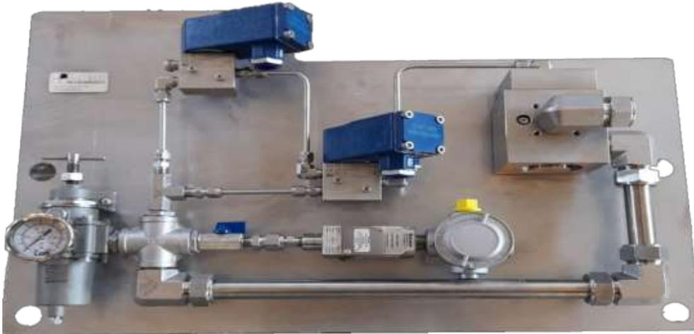
Such Skids are very common in process industries where they will operate ahead a control valve or ON OFF shut down valve or critical damper etc. Now although they are easy to build using standard components like pipes, fittings, small ball valves, solenoid valves and air operated valves etc but when they are to be serviced it becomes quite clumsy affair.
