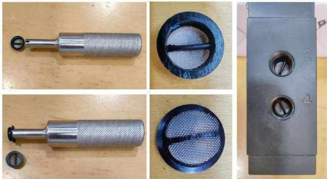
Above is an example of a protective screen guard. Now one may say what if my flow gets restricted due to the same ? Generally the open area of such screen is 36% higher than that solenoid valve orifice size i.e. if 6 mm is the orifice size then effective orifice of the screen is 7 mm. Thus effective area is  $49/36 = 36\%$  higher. For larger size this ratio even becomes larger as middle rib takes lesser space comparatively.
