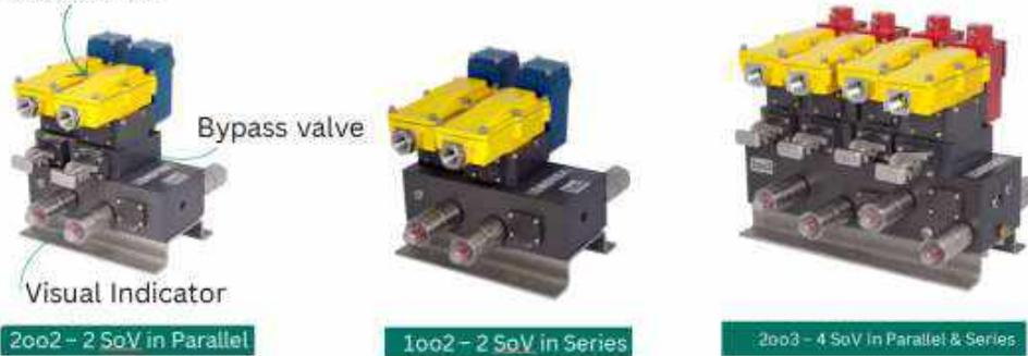
Thus upgraded version of 2002, 1002 and 2003 were introduced in the market which solved above mentioned problem. Here instead of using pressure switch, proximity switch was used to detect directly the solenoid valve component movement which then operated irrespective of inlet pressure supply from feeding valve. This system removed all drawback of the previous detection system and made it robust enough.
