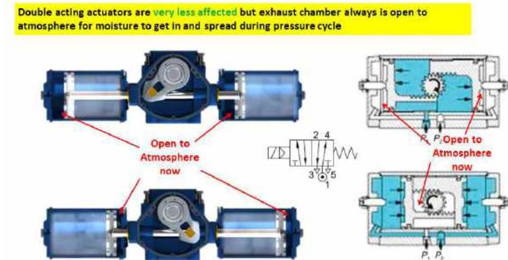
Even in Double acting solution once the particular section of the actuator is exhausted then it becomes open to the atmosphere where that portion gets exposed to atmospheric moisture or contamination which spread across the chamber during pressure cycle. Above pictures are of rotary actuators but this same problem persists even in leaner actuators i.e pneumatic cylinders
