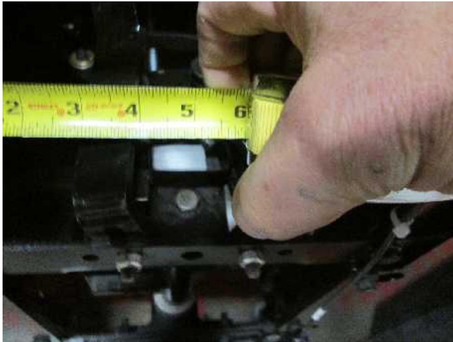
Be sure that the RUDDER ARM bisects the Rudder arm stop-bumper (Up and Down adjustment) Shim the Light Ball Sensor FRAME at the TOP two attaching bolts to RAISE the rudder arm or at the BOTTOM two frame attaching bolts to LOWER the rudder arm, so that the rudder arm BISECTS the rudder arm stop bumpers on a 45 degree angle.
