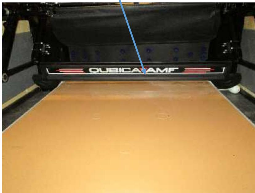
Step 7 – Crank/Run sweep back to HOME and tighten the 6 jam nuts loosened in Step 1. Run the sweep under power and adjust overall travel so the sweep travels rearward PAST the reference lines behind the 7 and 10 spots, BUT SHORT of the end of the Pindeck. Set all Guard positions for 1<sup>st</sup> and 2<sup>nd</sup> Guard and record positions in your manual.
