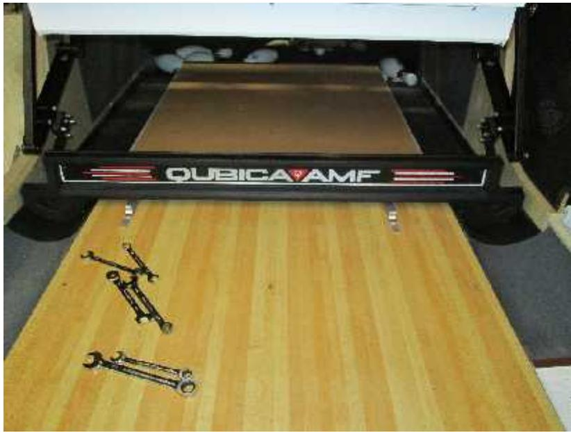
Loosen the bolt through the SLOT in the Triangular plate.
