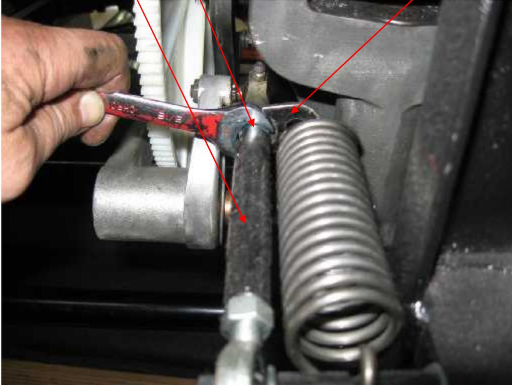
3. Make sure that pin seating rods are inward to within 1/8" of passing pinwheel cleats (7).
