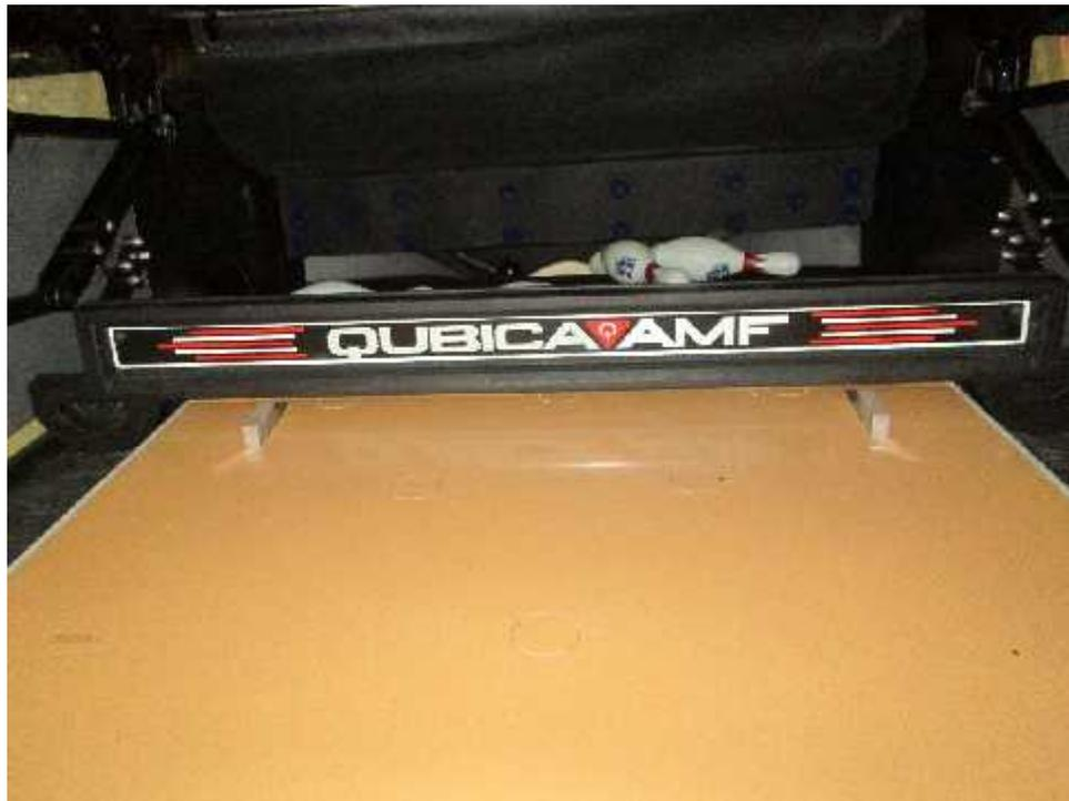
Step 4 – Adjust the sweep left or right to CENTER over pindeck. Gaps from pindeck to sweep should be near equal on both sides.
