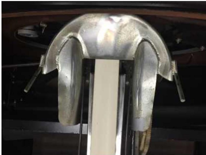
We "Balanced" all Distributors, setting the support weldment as low as possible and with a level Orientor Pan. We adjusted height to achieve  $\frac{1}{4}$ " clearance between the Front Belt Guide and the Durabin.
