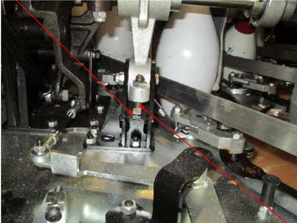
(First be certain that about 4 threads are showing between square head and housing). Check for any low or high hanging pins and adjust cups accordingly. Adjust the length of the SPOT ROD to achieve the 1/16" gap, between Square Head Stop Bolt and the Stop.
