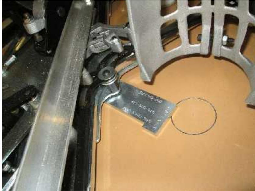
Adjust the CLEVIS length, so that the table is  $5/16$ " from the pindeck. We call this PARALLEL- $5/16$ ". The Table should be PARALLEL TO the pindeck AND  $5/16$ " from the pindeck. A bit higher than  $5/16$ " OK. Lower than  $5/16$ " not OK.
