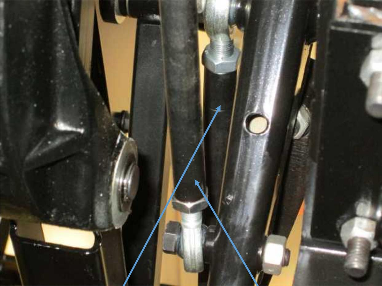
2 Jam nuts on the short travel rod and 2 each on the two long rods (7 pin side long rod not shown)
