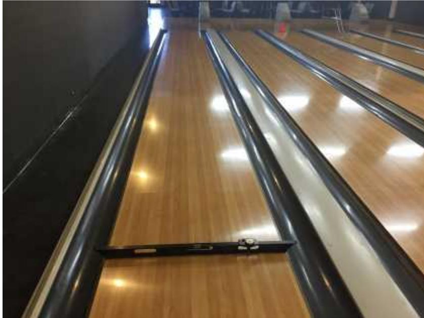
and inspected all ball lifts up front, and all Bowland X scoring, cap lighting, bumpers, front desk computer, and all furniture. They had one rope light with a broken plug on the cable side. I gave them part number (090-008-060) for a new cable. They had one bumper that didn't work. Red signal wire was loose in terminal board - fixed. The lanes were very good. I only needed to correct 9 places that were over .030" from zero. There were no places out of USBC Specification (.040").
