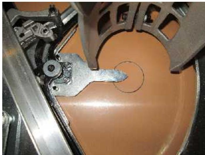
Check and adjust respot cells and cell-opening cam follower at this point if necessary. All cells should be fully open with a bit of "slop" in the rear fingers, as we discussed.
