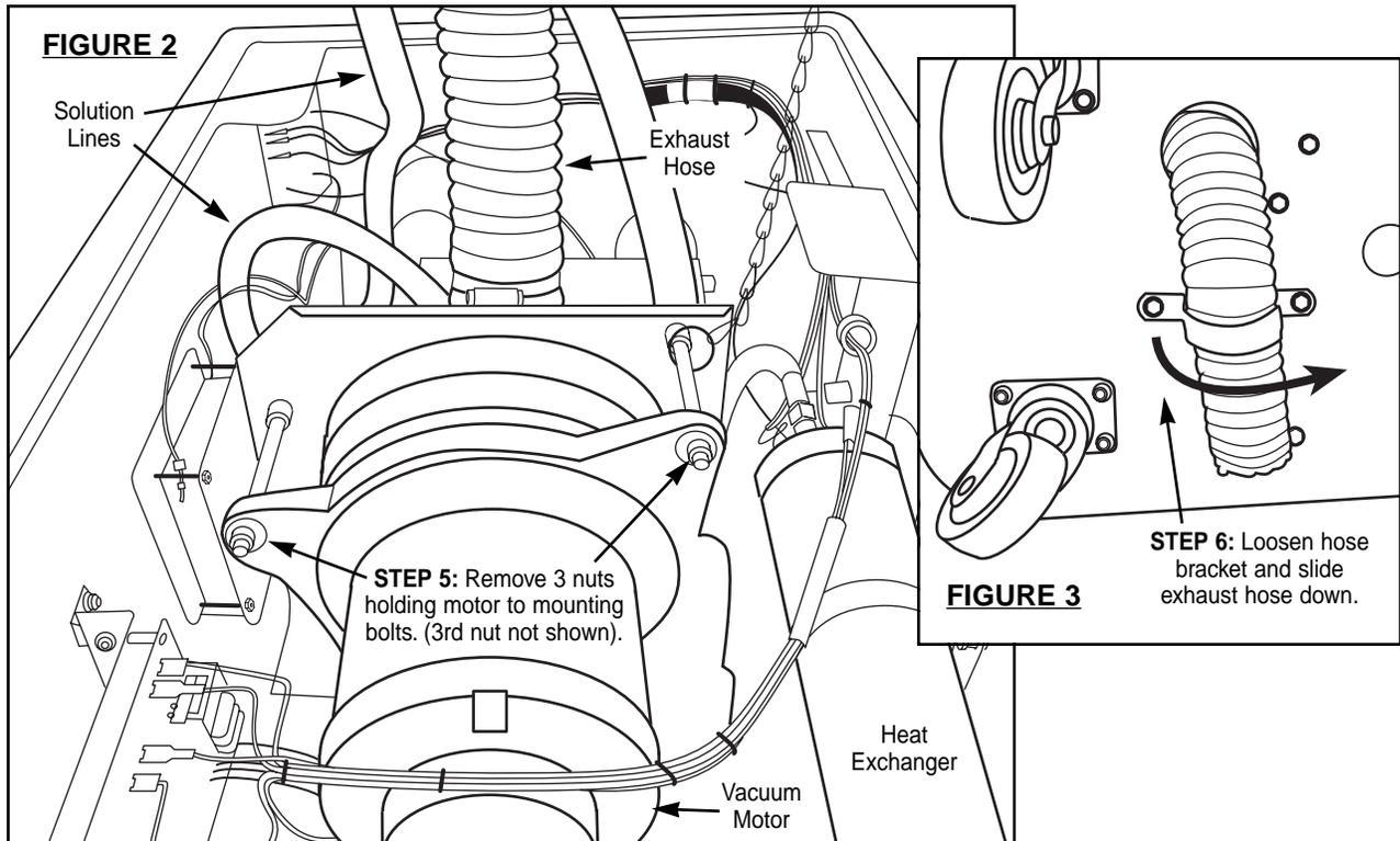
5. Remove the 3 nuts which hold the motor to the mounting bolts. See Figure 2 above.
