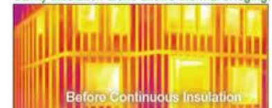
Adding exterior continuous insulation prevents heat flow through framing.
