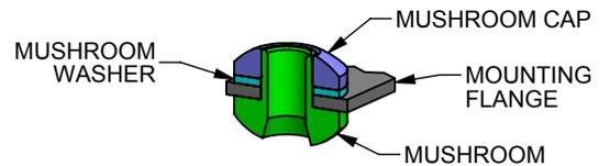
**FIG 2B: ALTERNATE INSTALLATION**
