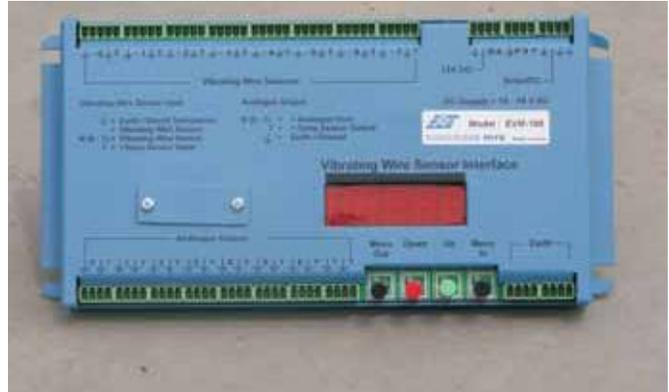
Figure 4: A SDI-12 Interface for connecting 8 vibrating wire sensors to a SDI-12 bus cable.
