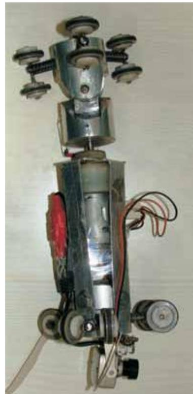
Fig-8: In-pipe robot for internal pipe inspection
