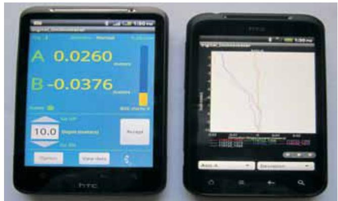
Figure 1: Mobile phones as readout unit (left) and on site analysis of movement profile (right).
