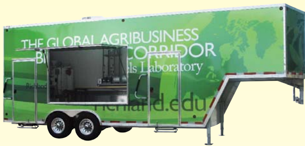
Two entry doors, back loading door, and one side mounted awning door
