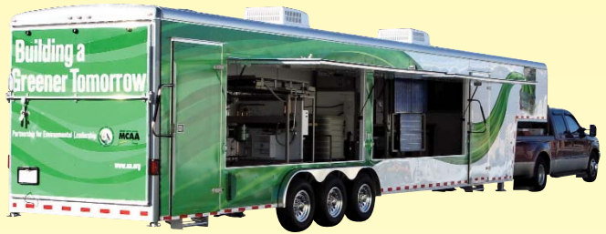
Two entry doors, back loading door, and two side mounted awning doors, and solar mounted roof panels
