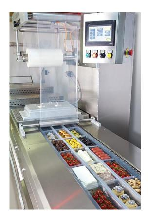
The MVZ - 150 offers you a more comfortable working environment with a servo motor for digital advancement, a state of the art PLC control system which allows for monitoring of parameters and necessary adjustments to be made easily and a touch screen operator panel with protection against external influences.
