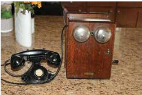
Old telephone with magneto generator
