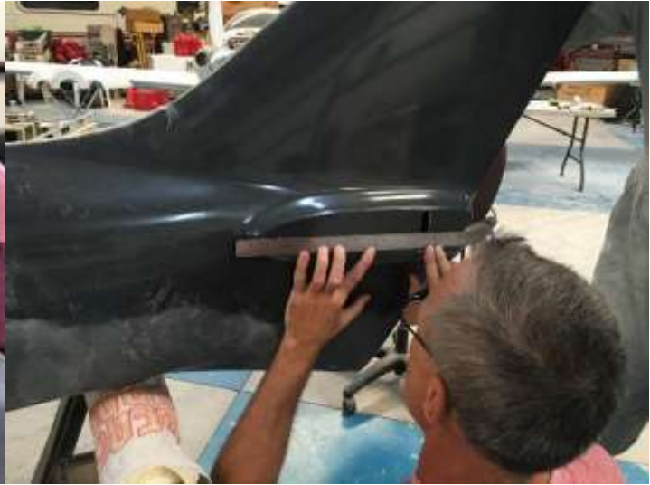
Setting the Angle of Incidence for the Stab
