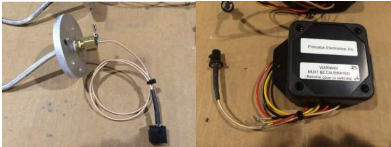
Close-ups of Probe Mount and Sending Unit
