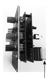
IMPORTANT: Power connection is red stripe downwards (facing the bottom of the unit) as shown in the picture above. Power diodes on the unit protect against reverse polarity connection.
