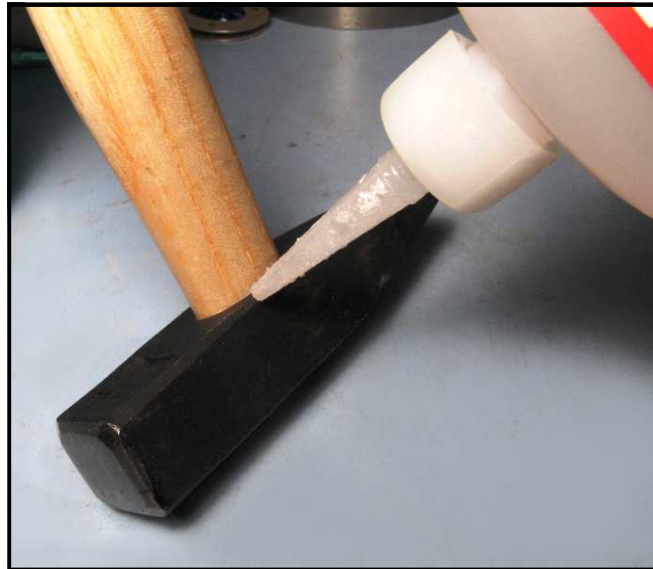
Applying Superglue to tighten the head to the handle.
