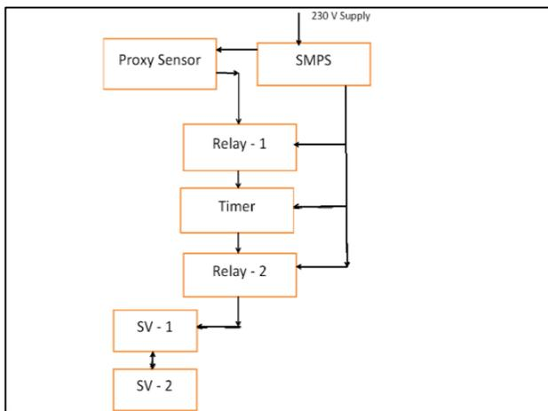
Fig.3 Block Diagram
