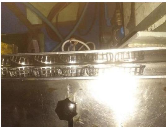
Fig .1 Bearings are stuck in Channel
