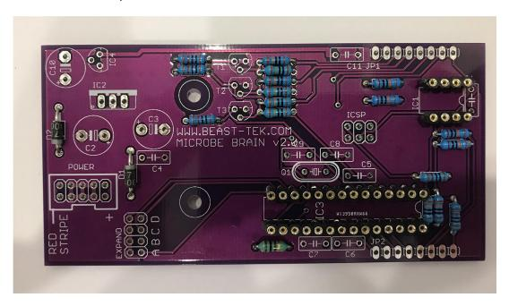
8. Install and solder 20 mhz crystal Q1
