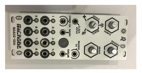
28. With the jack nut holding the front panel in place, give everything a wiggle around so that everything is sitting nicely. Take time and inspect that all the jacks and pots are sitting nicely. Now install washers and nuts on the four potentiometers and tighten (but don't over tighten, the pots aren't soldered and if you tighten them too much the pot leads will bend).
