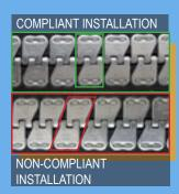
8. Take opposite belt side. Align i with the side already installed Min Record fastener.
