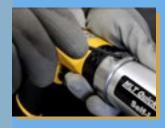
5.Turn the head for more comfortable use and tighten the clamping ring with an Allen key
