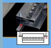
3.Insert gauge pin according to belt thickness. Tighten fastener and gauge pin with the locking cam (push side «F» for closing)
