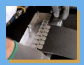
7.Slide the steel plate under the MR fastener and hammer the staple with the steel head hammer to close the Mini Record.
