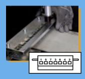
7.Press the trigger to activate the MLT Quick Driver (a few hits are enough), its punch will then hit and close the fastener. First close the strips on the edge (#1 and #2) using the MLT Quick Driver, checking the belt is still located against the fasteners guide. Then close a center strip (#3), and complete the installation by alternating the sides
