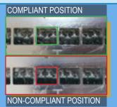
2.Place the Self-Lock® fastener in the installation tool so that each strip is under an opening in the device. The part with the hooks must be above
