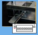
8.Unlock the cam (push «O» side) and take out the installed fastener. Take the other side of the belt and align it with the already fastened side. Mark the position of the second strip. Repeat from step 2
