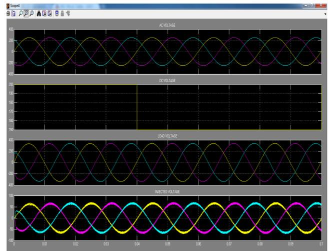
Fig. 8. Simulation result for DC Voltage Drop and the effect of DVR
