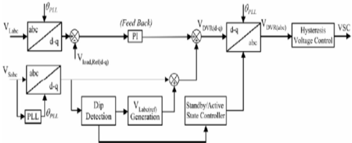
Fig. 5. Control Structure of DVR
