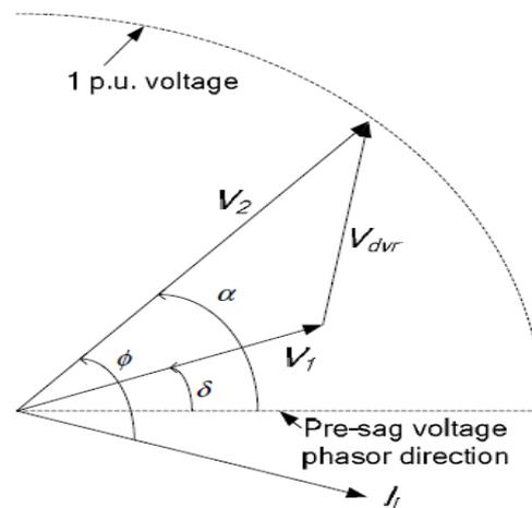
Fig. 1. Phasor Diagram of power distribution system during a sag
