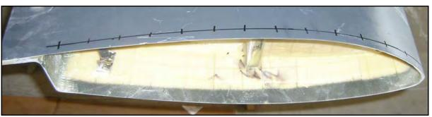
8. Use the photo below as a reference for setting up some items that will help fitting the wing tip. Items need are: 2 foot piece of scrap angle aluminum. At least a 4 foot piece of scrap angle aluminum, weighted bag (shot works), clamps and clecos.
