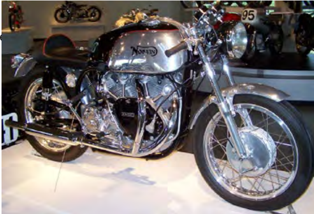
A Norton Featherbed with a Vincent engine. Photo Credit: John H Glimmerveen Licensed to About.com
