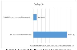
Figure 5: Delay of MOSFET based Comparator and GNRFET based Proposed Comparator
