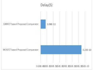
Figure 8: Delay of MOSFET based Proposed Comparator and GNRFET based Proposed Comparator
