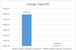
Figure 7: Average power of MOSFET based Proposed Comparator and GNRFET based Proposed Comparator The graph figure 7 diagram shows the Average power of MOSFET based Proposed Comparator and GNRFET based Proposed Comparator. here we can see the average power is less in GNRFET based Proposed Comparator and high in MOSFET based Proposed Comparator.
