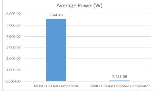
Figure 6: Average power MOSFET based Comparator and GNRFET based proposed Comparator
