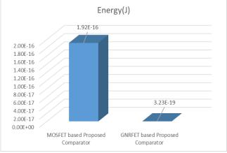
Figure 9: Energy of MOSFET based Proposed Comparator and GNRFET based Proposed Comparator
