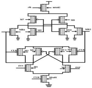
Figure 1:dynamicdouble-tailcomparator using GNRFET
