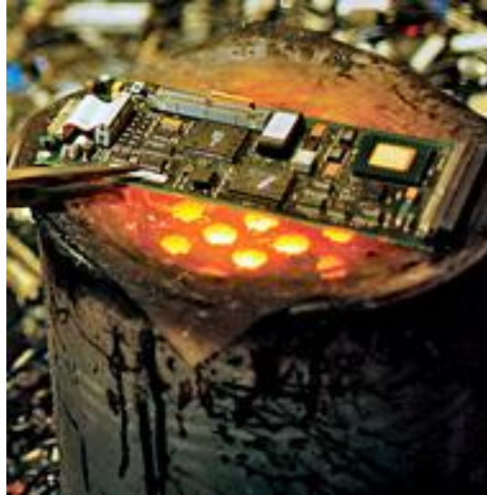
PCB Heating Technique for Removal of Used ICs to be Resold on Counterfeit Market
