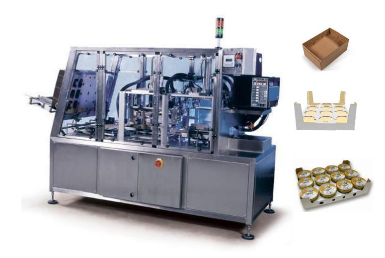
$TR-201^{TM}$  automatic tray erector that erects trays in a triangle corner post formation.
