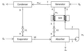
Hence to utilize the exhaust gases and waste heat from an engine the vapor absorption refrigerant system can be put into practice, which decreases the cooling water temperature. That leads to proper cooling of diesel engines walls there by increases the overall performance of diesel engine and also reduce the problem of leaking of cooling water which is caused by the over heating of engine parts. **Advantgaes -**
