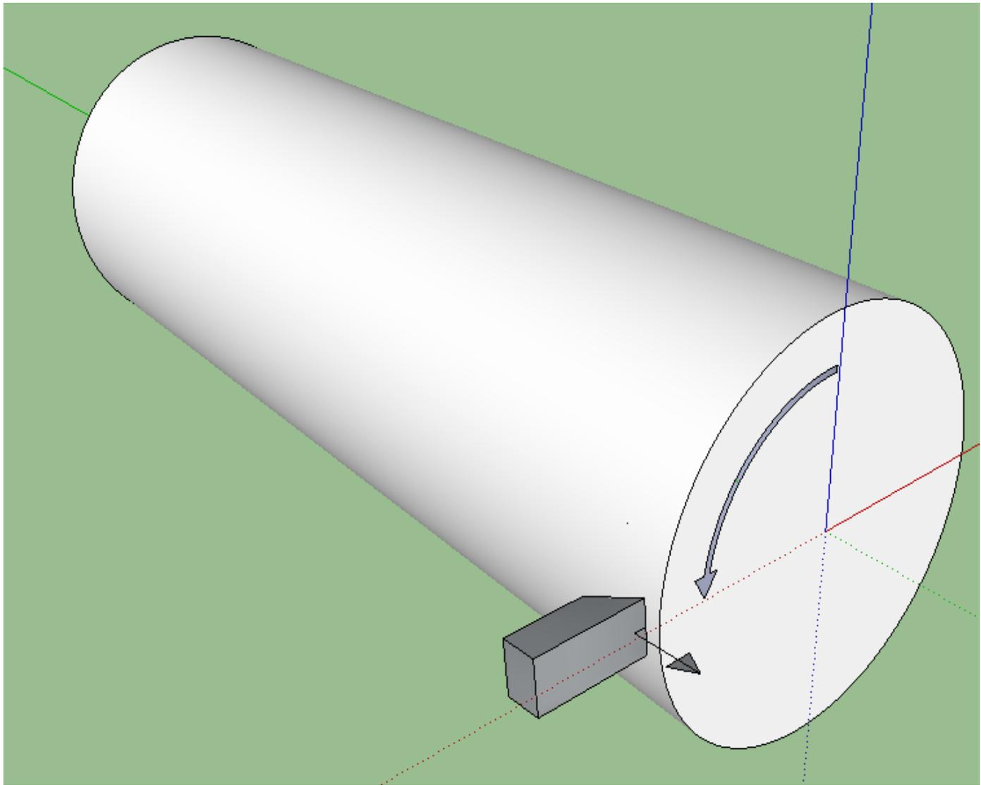
First, you have to consider the grain direction. You should always go WITH the grain, going against the grain causes tear out.
