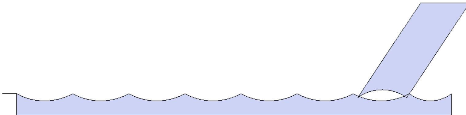
The long bevel and hollow grind will rise and fall with the washboard tool marks
