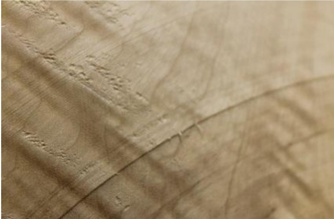
By closing the flute, the gouge will slice the wood fibers with the nose radius instead of just cutting them. Notice that the cutting edge is almost parallel to the rotation of the wood. Again, note how I rub the bevel to control the depth of cut. Slicing Cut
