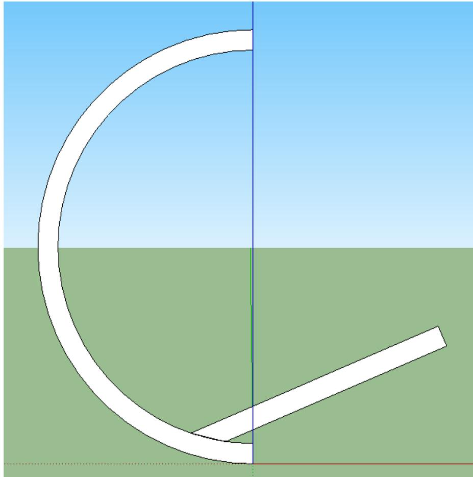
The tool is  $\frac{1}{2}$  the way through the cut and notice how close it is to the side of the bowl
