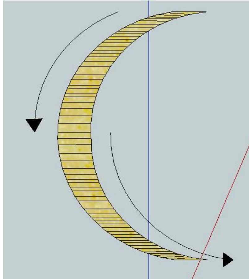
I use the gouge with the flute about half open to rough turn. It may be hard to see, but I am rubbing the bevel to control the depth of the cut. Shear Cut.
