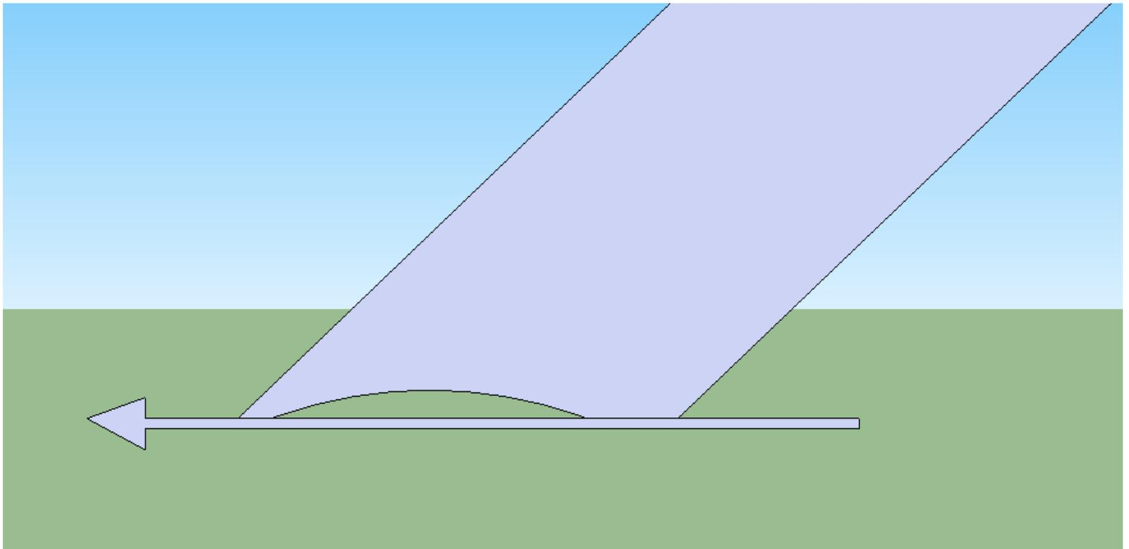
Much less used is a convex grind bevel, but it has an advantage; it works like a carving chisel. It wants to move up and out of a cut.
