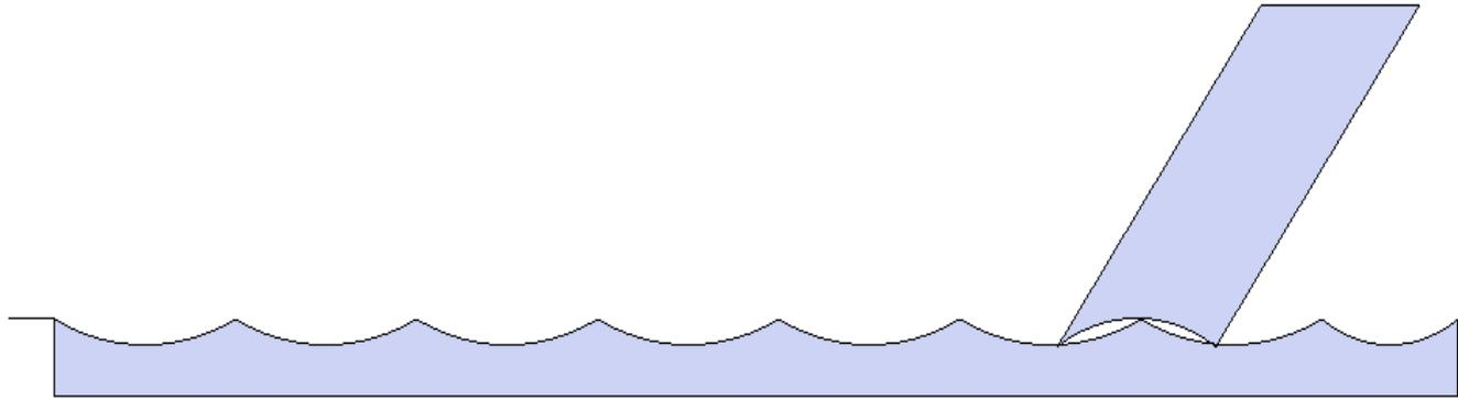
Grind a micro bevel (clearance) on the
