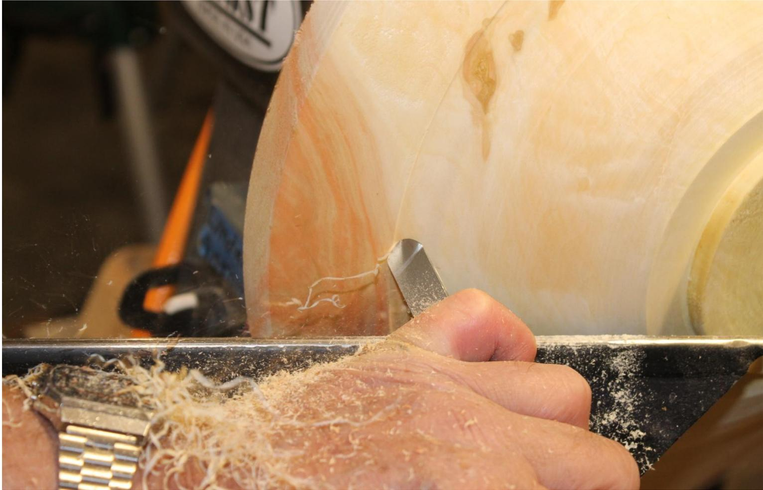
By using the cutting edge almost parallel with the rotation of the lathe, The finish is smooth.
