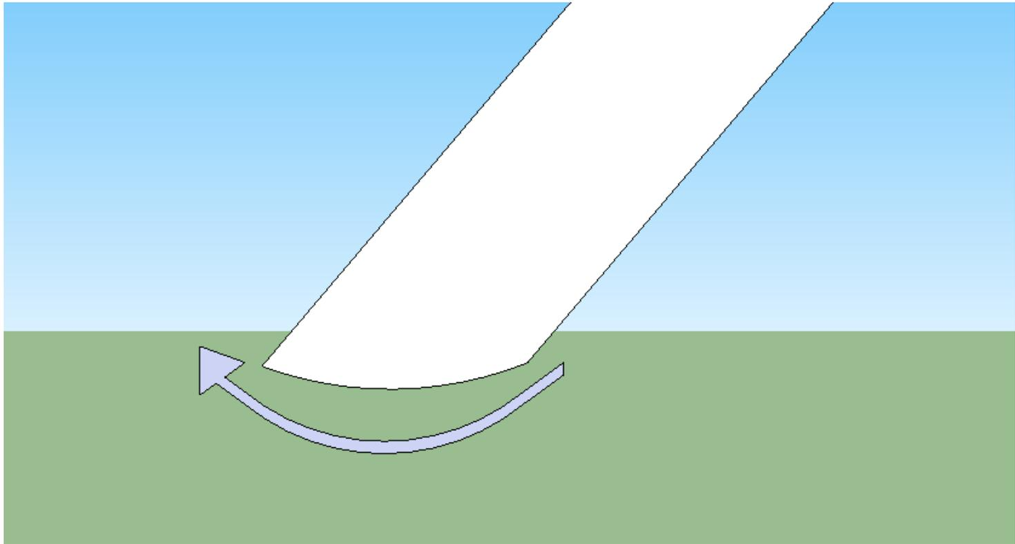
(Exaggerated hollow grind bevel)
