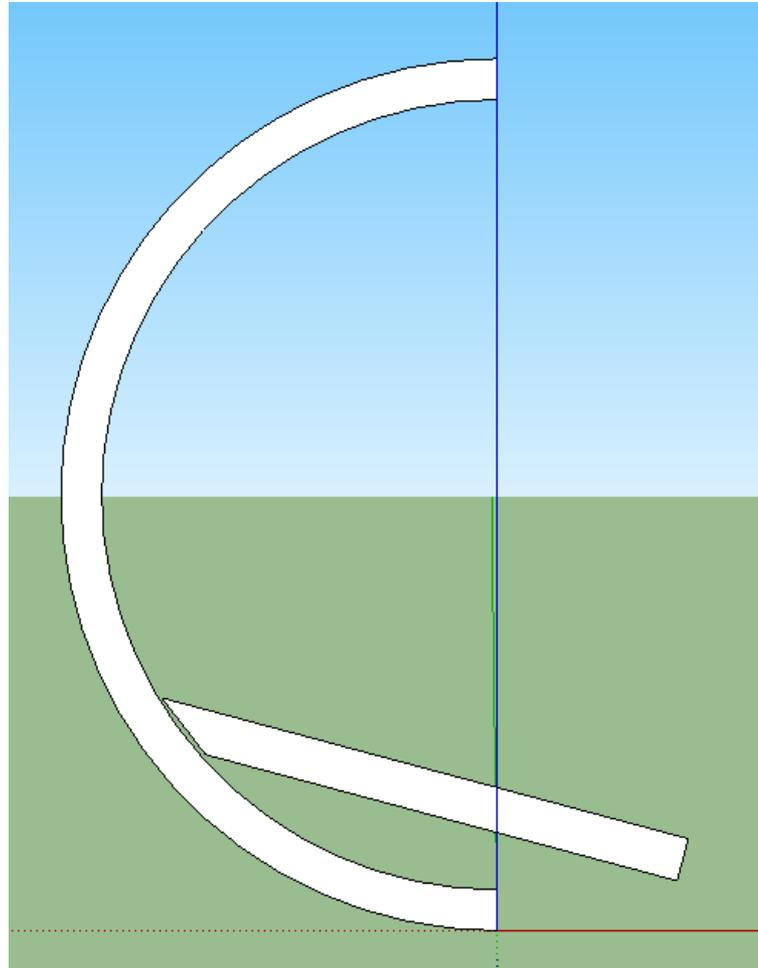
Now the tool is almost to the bottom of the bowl and is rubbing the side of the bowl. It can not complete the cut
