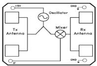
Fig 3: Block diagram of Radar Module
