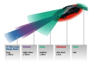
Fig 1 : Range of different sensors
