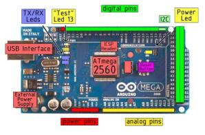
Fig 2: Arduino prototype Development Board
