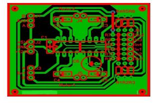
Fig 5: Final Printed Circuit Board
