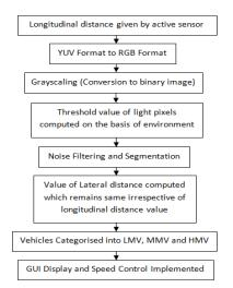
Fig 6: Flow diagram of software implementation
