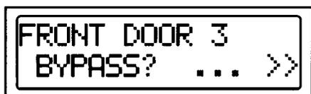
Press **SELECT** to bypass that sensor. The sensor will be bypassed for this arming only. If there are more violated sensors, the system will repeat this process.
