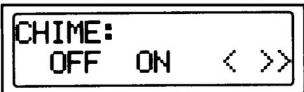
A rectangular display screen with a double border. The text inside reads "CHIME:" on the top line and "OFF ON < >>" on the bottom line. The word "OFF" is flashing.
