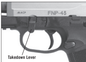
Rotate the takedown lever downward.
