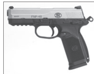
Hammer cocked for single-action firing
