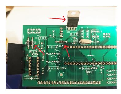
Once soldered, trim off the component legs using side cutters.
