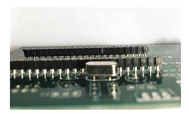
Now solder the remaining IC pins and crystal.
