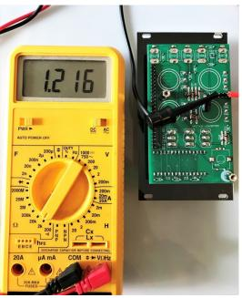
If the resistance is 0 or the continuity test registers a connection, then there is a short circuit somewhere. Inspect the board visually, if you cannot locate a short then there may well have been too much solder applied to the SPST which caused a short between a switch body and the PCB.
