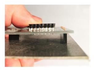
Only solder 2 pins on each strip, then turn the board over to inspect and make sure the header strips are seated at a right angle and that they are flush with the PCB board. If required, the header strip can be adjusted by heating one joint at a time and gently moving the header strip into the correct location.
