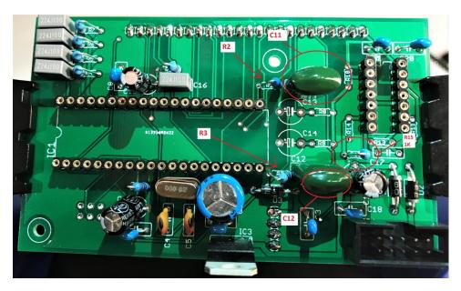
Install the two 4.7uf electrolytic capacitors C13 and C14. Install the six 10K ohm resistors R8, R9, R10, R11, R13 and R14. Solder and trim leads.
