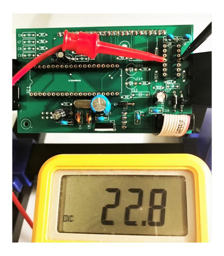
IC2 – connect the positive probe to pin 4 and connect the negative probe to one of the ground pins on C20 or C21 located directly above IC2.
