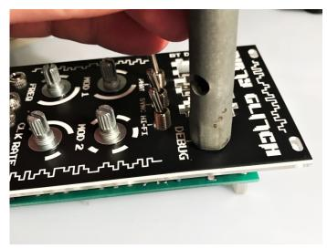
Place washers and nuts onto the 4 pots. Tighten the nuts, again using a tube spanner or ring spanner to avoid scratching the front panel.
