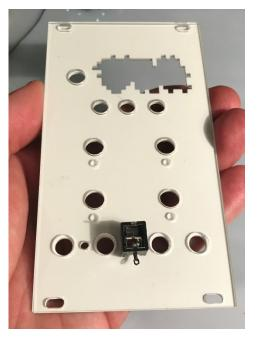
Once all five jacks are installed, make sure that the pins are all straight and make sure the jack bodies are aligned nicely. Bend the ground connector on each of the jacks at approximately 45 degrees as per the photos.
