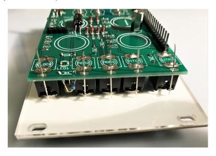
Unscrew the 10mm stand-off located in the upper corner of the PCB. Insert the 1mm nylon washer onto the screw and replace the 10mm stand-off on top of the washer.
