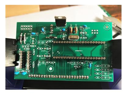
Install and solder the  $2 \times 100$ uf electrolytic capacitors (C1, C19) followed by the 10uf electrolytic capacitor (C15) and the 470uf electrolytic capacitor (C22).
