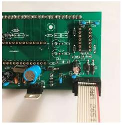
Once the IDC socket orientation has been confirmed using the power cable, solder the remaining pins.
