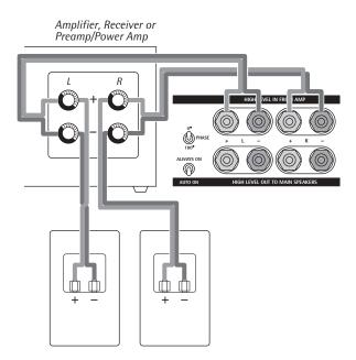
The other method is to connect the amplifier to the main speakers and then run extension wires from the main speakers to the ICS Sub 24.
