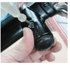
While pinching the housing together and making sure the switch and button are in position, remove the alignment tool. The long bolt can be easily passed into the housing and fixed with the hex nut underneath.
