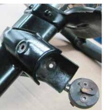
Now place the button over the end of the switch and into the housing's rim, as shown in the next photo. A helpful hint is to use a small tool with a shaft the size of the long bolt, like a punch, to align the switch to the holes in the housing. The switch has two matching holes that the long bolt must pass through and out of to secure the housing to the column.
