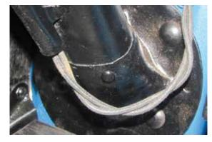
The next step is to trim the two wires and attach them to the switch contacts. Applying a bit of solder to 'tin' the bare wires makes it easy to form a loop to secure the wires under the attachment screws.
