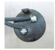
Now gently expand the switch housing and place it around the steering column, noting that the lower edge has the formed outlet for the wires coming from under the steering column. Position the wired switch contact into the spread-apart housing and gently align the two wires so they will pass out of the formed lower edge; otherwise, the wires can bind and keep the housing from closely completely around the steering column.
