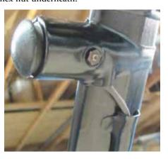
The restored horn button is now mounted on the steering column. Attach the ends of the two horn wires to complete the install. The longer wire goes to the horn positive (+) terminal. The shorter wire is placed under the screw at the firewall terminal of the generator/ammeter wire (+) (yellow/black tracer) for the 6 volt DC horn; or at the magneto terminal (red wire) (+) for the magneto AC horn.
