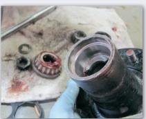
Clean all the bearings in preparation to inspect and regrease them. All the taper bearings should be clean and without cracks or excess wear. Also inspect the inner races for cracks, as well as the wheel hubs.
