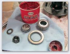
Grease well, including the inner races, and slather gobs of grease into the hub cavity, too. Refit the inner bearing, topping it off with the dust shield. The hub can then be tapped with a mallet or wood block back onto the spindle. Alternately, you can fit the dust shield over the spindle and press on the inner bearing, driving it with a sleeve tool that doesn't impact the taper bearings before fitting the hub. This is needed at times when the press fit is really nice on the spindle surface.
