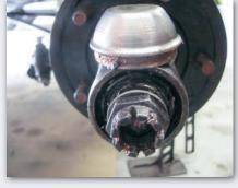
the nut and the toothed lock washer. (Note left hand threads on right front [passenger], right hand threads on left front.)
