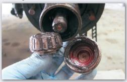
Remove the wheel hub, as the inner bearing race should be a light press fit on the spindle. A puller is handy for removing the hub. Remove the inner bearing by tapping it out carefully from the inside with a long thin rod. The dust cap normally falls away as the inner bearing is driven out. In the photos to the right, the red grease is still in good shape but the bearing should be cleaned well to inspect it, too.
