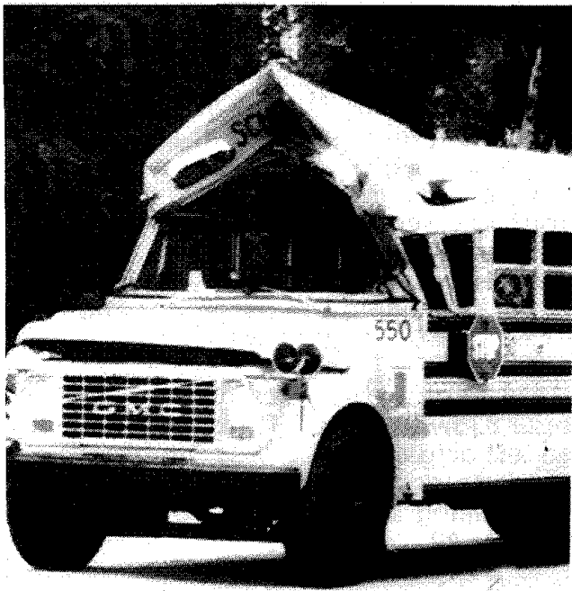
Figure 4.--Left photograph shows damage to Miami, Florida, schoolbus. Right photograph shows interior damage caused when the truck wheel penetrated the front windshield of the bus.
