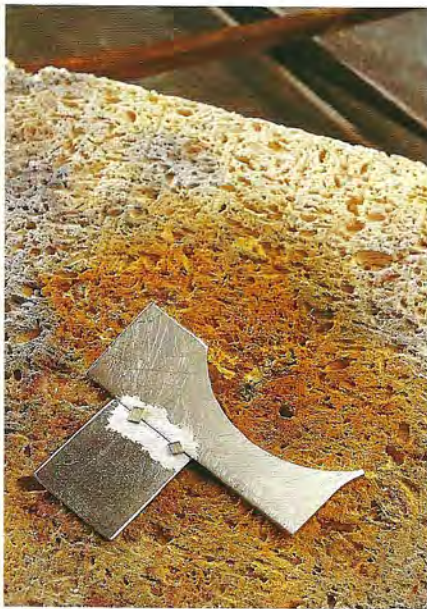
Chips of solder span a fluxed joint.
