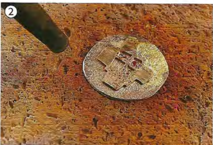
2 ...then set that piece onto another. Heat the whole assembly until the solder flows.
