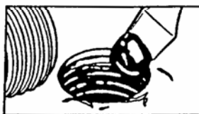
Step 5) Fill damage with FORM-A-THREAD™ compound.
