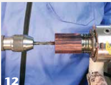
12 Drill into the base section with a \frac{3}{8} " bit, deep enough for the spin-top handle to go all the way in.
