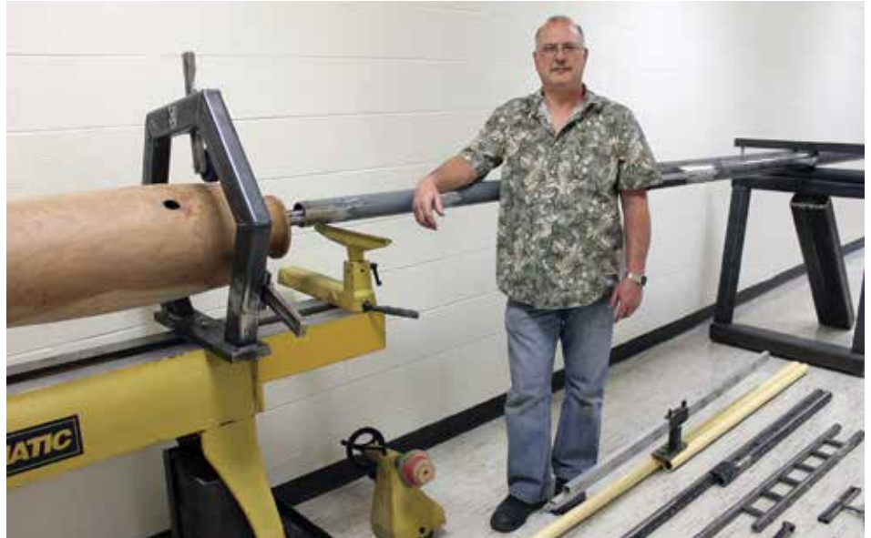
Lyndal Anthony with his well-researched boring bar outfit made for very deep hollowing.
