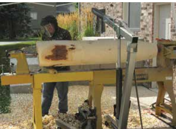
Before hollowing, the author turns the workpiece between centers to shape the outside of the vessel. Note the engine hoist used to help position the log section. Prior to actual turning, he uses a portable power planer to knock down the high spots and balance the piece better.
