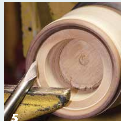
5 Form a bead on the walnut accent wood. The author refines the bead using a spindle gouge in shear-scrape mode. With the flute facing the wood and the handle down, drag the lower cutting edge carefully around the bead.
