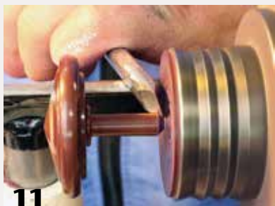
11 The author uses a skew chisel to make small "V" cuts until the top is parted off.
