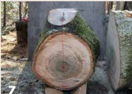
7 As with the straight-grain log, the crotch section is cut apart vertically. Transferring the location of the pith to the top of the log on both ends, as well as drawing the vertical line to the pith, guides the central cut.
