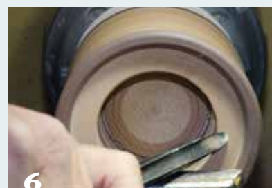
6 The author cleans up the narrow maple area inside the bead with the lathe running in reverse direction.
