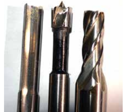
From left: router bit, Forstner bit, and milling cutter. The centerpoint on the Forstner bit effectively limits the potential depth of a stopped hole in thin wood.
