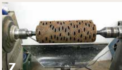
7 A banksia pod mounted between centers with its core running parallel to the lathe bed. Tenons are formed on the ends for holding in a four-jaw chuck.
